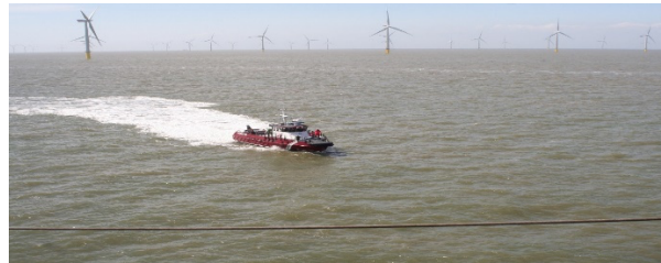
Vessel to standby 100m from the turbine until called in by rescuer
